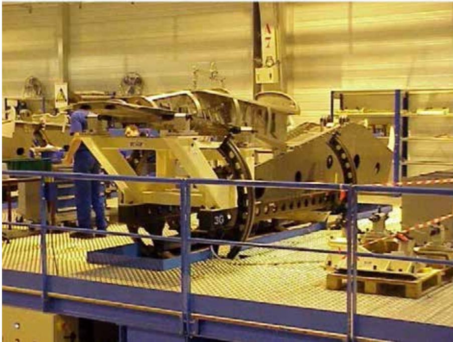
Figure B-1 Building a Pylon
