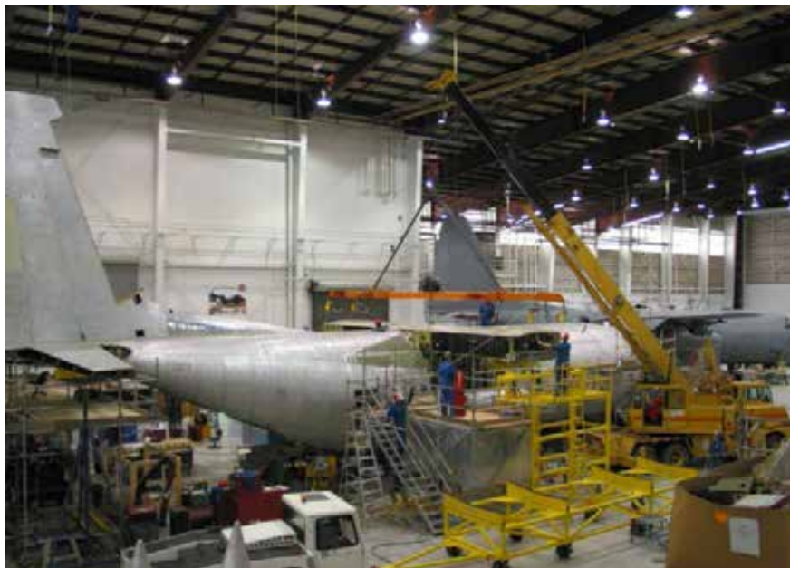
Figure A-2 Placing a C-130 Centre Wing
