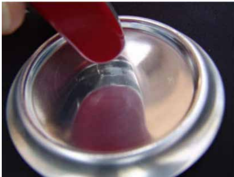
Figure 5 Verifying the Polish
